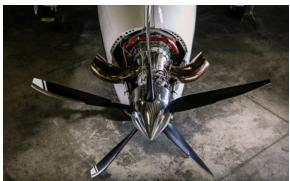
The strength of **MT propellers** is based on tests, simulations and calculations per CS-P-330 (EASA Requirement) or FAR 35.24 (FAA Requirement). The **MT propellers** have at least a 10 times safety factor built into the blades which is why there has never been a blade failure in more than 110 million flight hours with more than 60,000 blades flying. If the Hartzell propeller were 10 times stronger that would imply a 100 times safety factor!
